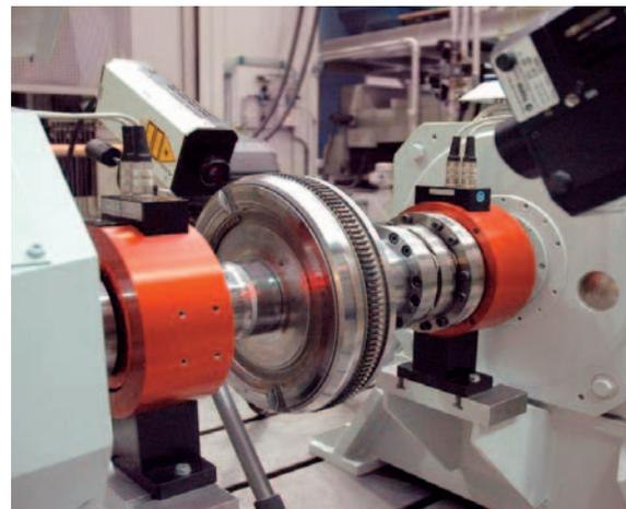
Figure 2: Dual mass flywheel on the test rig.
