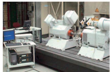
Figure 1: Dynamic test rig for drive elements.
