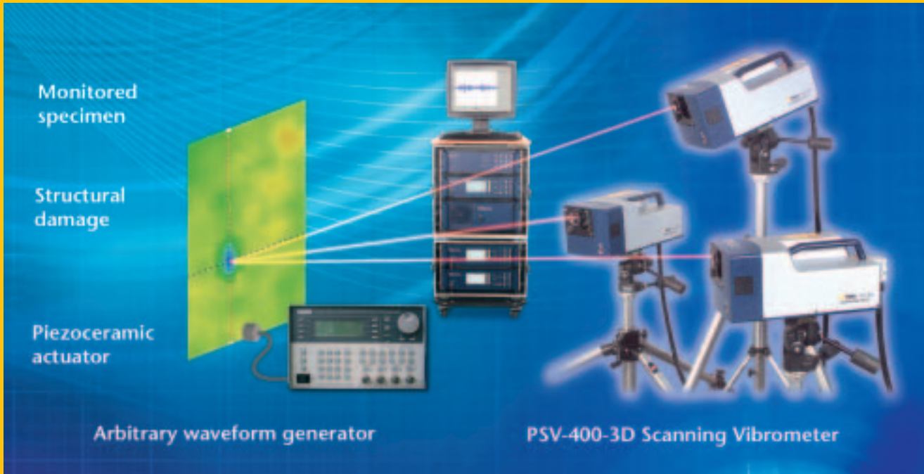
Figure 1: Experimental arrangements for Lamb-wave damage detection using 3-D laser vibrometry as a receiver
